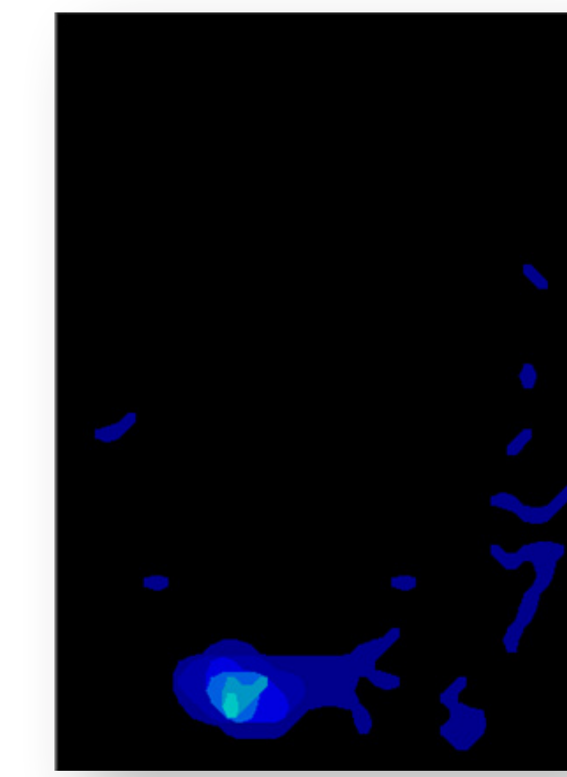
Figure 7d – Tekscan under 700N load at 4mm of distraction
